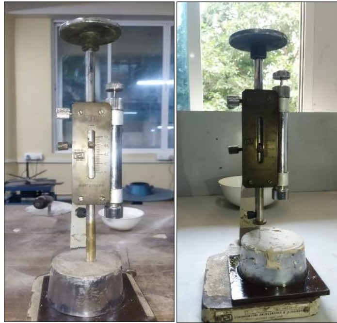
Figure 4 Initial and final setting time test
