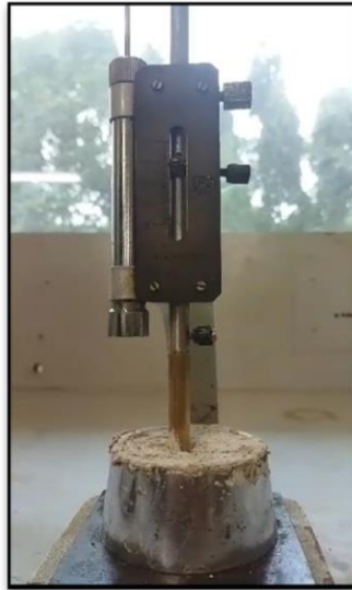
Figure 3 Standard consistency test
